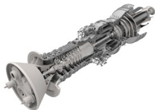
Exhibit 1: Cross Section of a Mobile Natural Gas Turbine, Showing Turbine Blades
