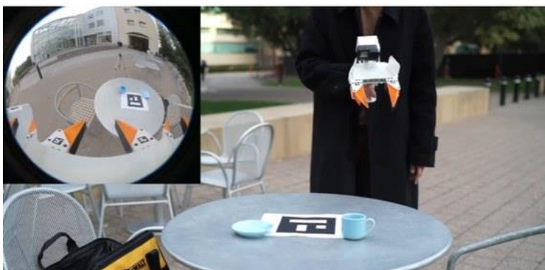
Fig. 5: UMI Policy Interface Design. (b) UMI policy takes in a sequence of synchronized observations (RGB image, relative EE pose, and gripper width) and outputs a sequence of desired relative EE pose and gripper width as action. (a) We synchronize different observation streams with physically measured latencies. (c) We send action commands ahead of time to compensate for robots' execution latency.
