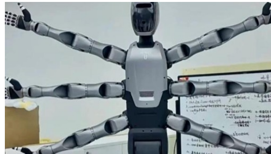
Midea Robot Ultra, a wheel-based 6-arm humanoid, working in washing machine production line
