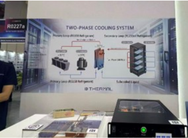
图表 3: Kaori two-phase cooling system
