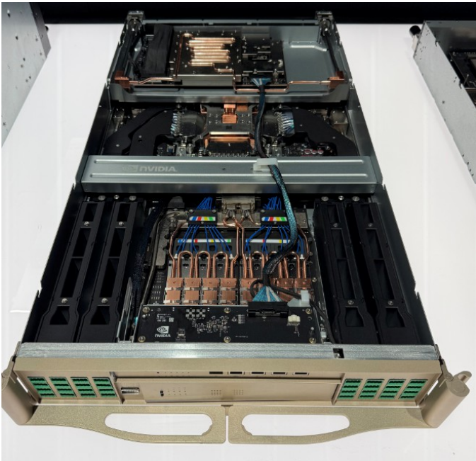
Figure 5: Nvidia's Spectrum-X SN6810 CPO switch
