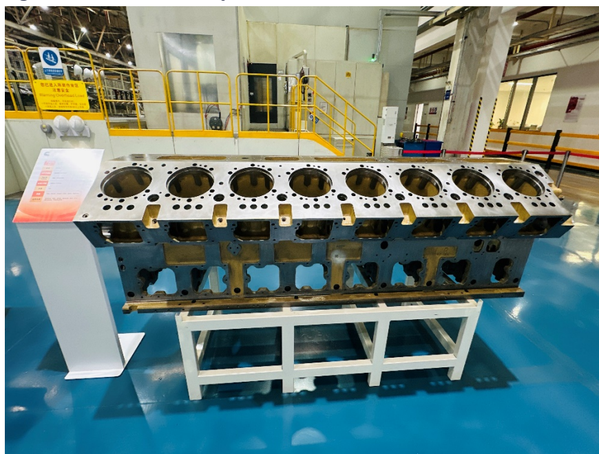
Figure 5. CQ Cummins 50L cylinder block
