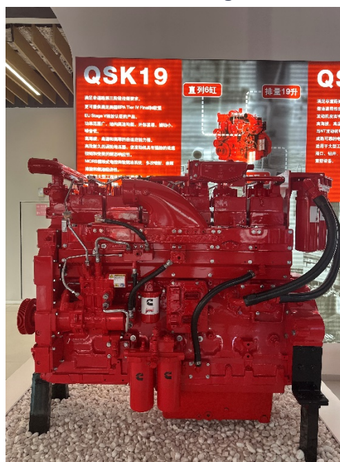
Figure 2. CQ Cummins Q19 diesel engine
