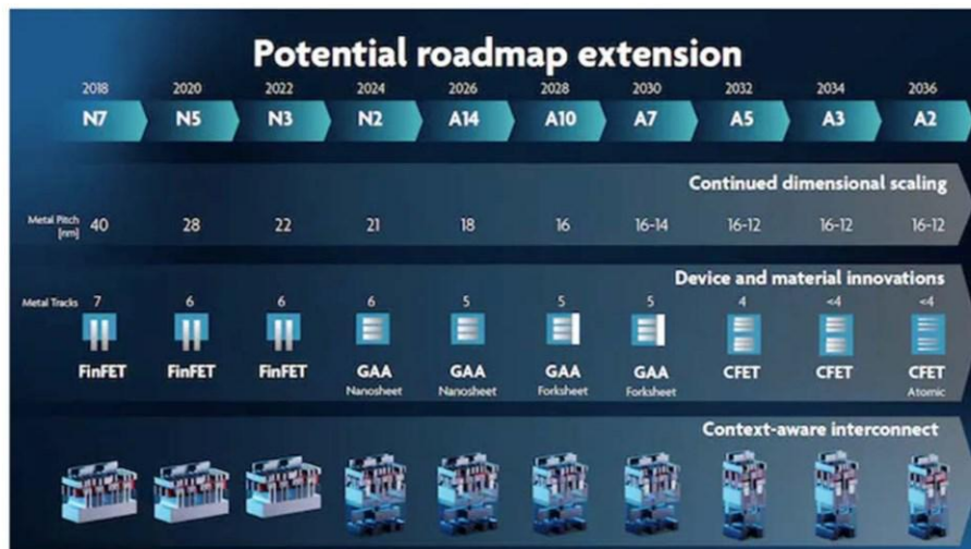
Fig. 72: Semi logic nodes roadmap
