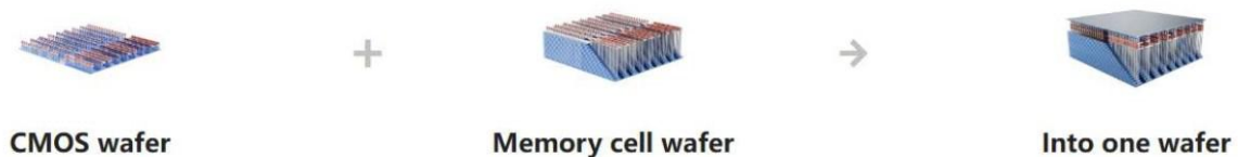
Fig. 183: The wafer bonded NAND wafer input vs output
