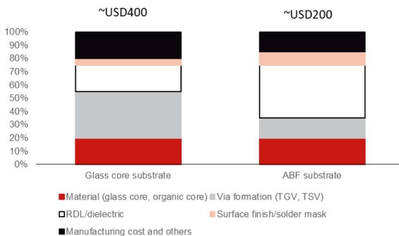
Fig. 102: Potential BOM cost of glass core substrate vs ABF substrate
